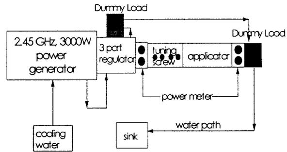
**Figure 8.2** A single mode microwave system. A magnetron is used to generate 3000 W of power at a frequency of 2450 MHz. Reflected waves are prevented from damaging the generator by a regulator connected to the power source. A tuning screw matches the impedance between source and load, and a power meter monitors forward and reflected power. Welding is performed in the applicator, and dummy loads dissipate power by converting transmitted energy into heat.
