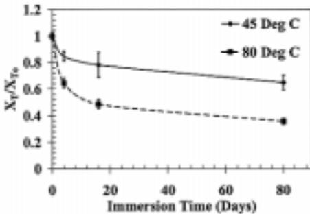
Figure 5. Cross-ply tensile strength normalized to unaged 25°C strength versus time of immersion.
