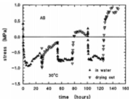
Figure 4. Development of residual stress in an AB coating 212  $\mu\text{m}$  thick during wet/dry cycling at 30°C (48 h period).
