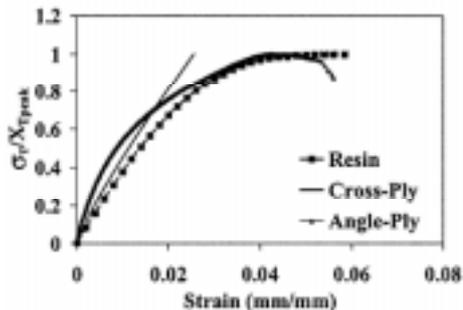
Figure 1. Tensile stress/strain curves normalized to peak tensile strength.
