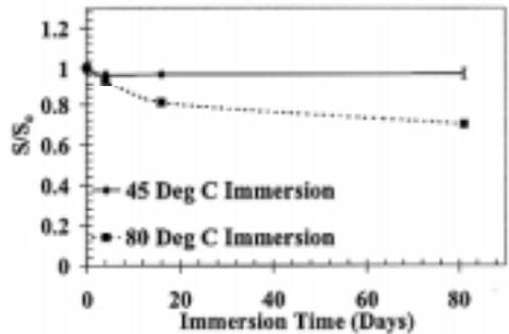
Figure 6. Angle-ply shear strength normalized to unaged 25°C shear strength versus time of immersion.
