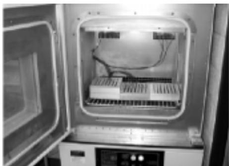
Figure 2. Freeze-thaw conditioning chamber.
