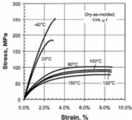
Figure 5a. Effect of temperature on tensile behavior of dry-as-molded nylon 6 (33% glass fiber).
