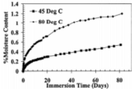
Figure 4. Pultruded vinyl ester E-glass laminate % moisture content (MC) versus time of immersion.
