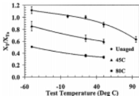
Figure 7. Comparison cross-ply tensile strength relative to test temperature for specimens unaged and immersed for 80 days in 45°C and 80°C water.
