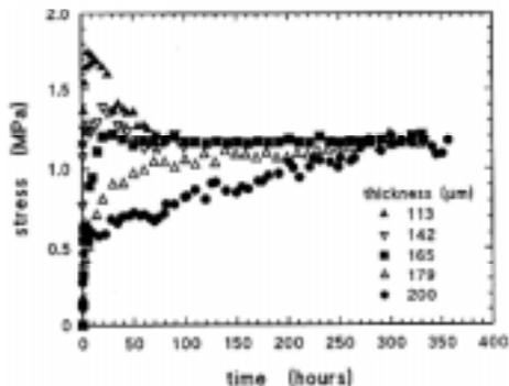
Figure 1. Development of residual stresses during solvent evaporation in AA coatings of different thickness.
