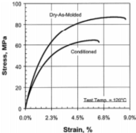
Figure 2c. Effect of moisture on tensile behavior of reinforced nylon 6 (33% glass fiber) at elevated temperature.
