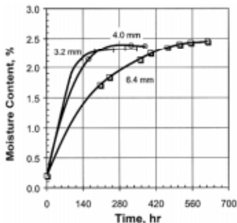
Figure 1. Moisture absorption vs. time for 33% glass fiber reinforced nylon 6. The number in mm by each curve indicates the thickness of the samples.<sup>5</sup>
