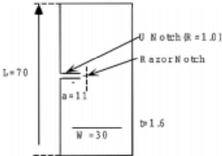
Figure 1. The shape of the specimen for ECT tests.
