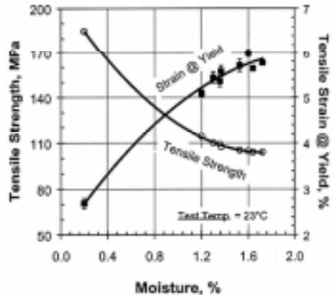
Figure 3. Effect of moisture on tensile properties of reinforced nylon 6 (33% glass fiber); tensile strength and strain at yield vs. moisture at room temperature.
