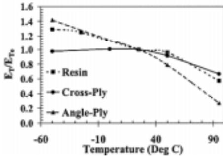
Figure 3. Tensile modulus normalized to room temperature unaged modulus
