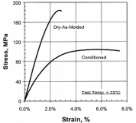
Figure 2b. Effect of moisture on tensile behavior of reinforced nylon 6 (33% glass fiber) at room temperature.
