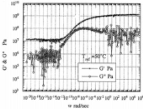
Figure 2. Master curve for Epoxy B at 50°C.
