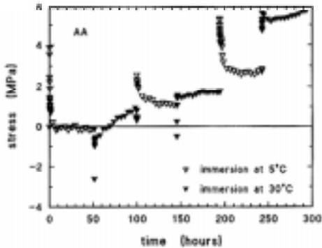
Figure 6. Development of residual stress in an AA coating 252  $\mu\text{m}$  thick during wet (5°C)/dry (room temperature) cycling (96 h period).
