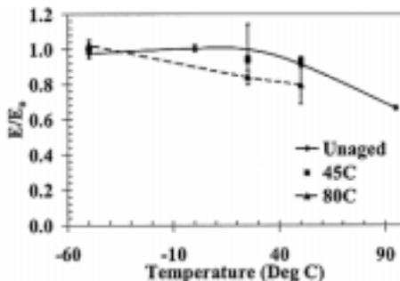
Figure 9. Comparison cross-ply tensile modulus relative to test temperature for specimens unaged and immersed for 80 days in 45°C and 80°C water.
