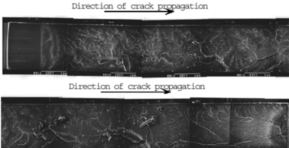
Figure 6. The SEM image of the fracture surface of the ECT test shown in Figure 2.
