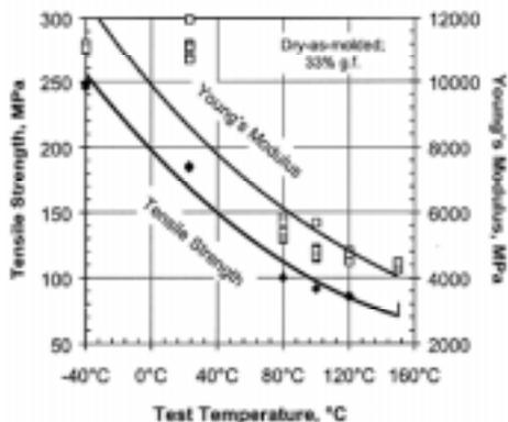
Figure 6. Effect of temperature on tensile strength and Young's modulus of dry-as-molded nylon 6 (33% glass fiber).
