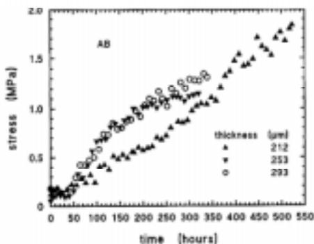
Figure 2. Development of residual stresses during solvent evaporation in AB coatings of different thickness.
