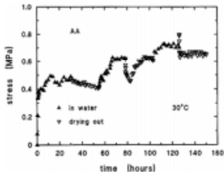
Figure 3. Development of residual stress in an AA coating 165  $\mu\text{m}$  thick during wet/dry cycling at 30°C (48 h period).
