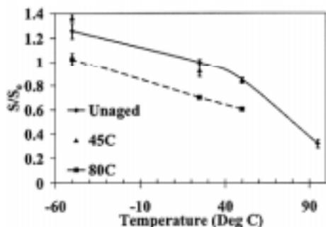
Figure 8. Comparison angle-ply shear strength relative to test temperature for specimens unaged and immersed for 80 days in 45°C and 80°C water.
