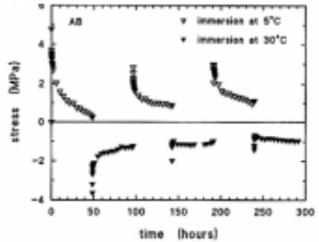
Figure 7. Development of residual stress in an AB coating 235  $\mu\text{m}$  thick during wet (5°C)/dry (room temperature) cycling (96 h period).
