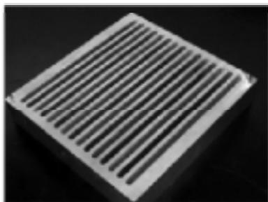
Figure 3. Unloaded sample freeze-thaw tray.
