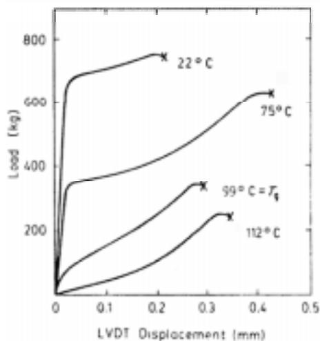
Figure 1. Illustration of loss in strength for an epoxy approaches  $T_g$ .<sup>2</sup>
