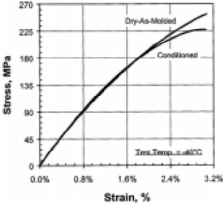
Figure 2a. Effect of moisture on tensile behavior of reinforced nylon 6 (33% glass fiber) at low temperature.
