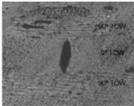
Figure 1. Typical crack in toughened vinylester composite (0.24mm by 0.08mm).
