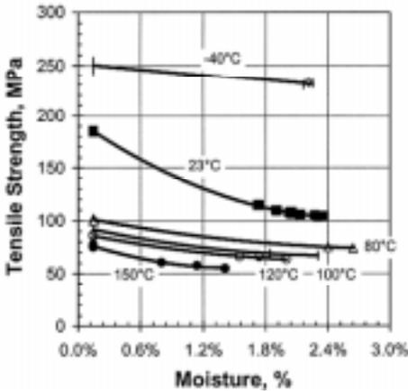
Figure 7. Impact of temperature and moisture on tensile strength of reinforced nylon 6 (33% glass fiber).
