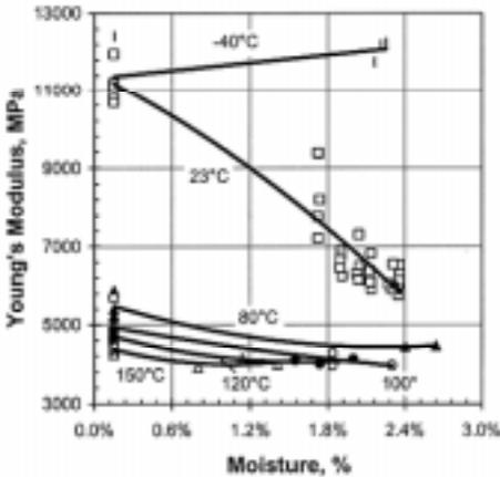
Figure 9. Impact of temperature and moisture on Young's modulus of reinforced nylon 6 (33% glass fiber).
