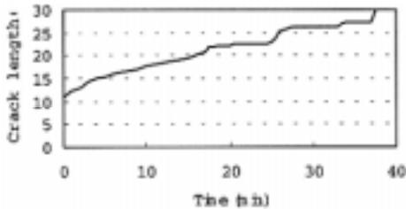
Figure 2. The ECT test result in surfactant A for  $\sigma = 8.2 \times 10^5$  Pa at 23°C.
