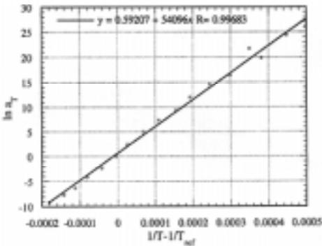
Figure 3. Arrhenius plot for Epoxy B activation energy determination.
