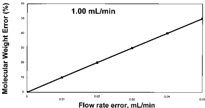
**Figure 16** Effect of pump flow rate precision. Each 1% error in GPC flow rate results in a 10% error in molecular-weight value.
