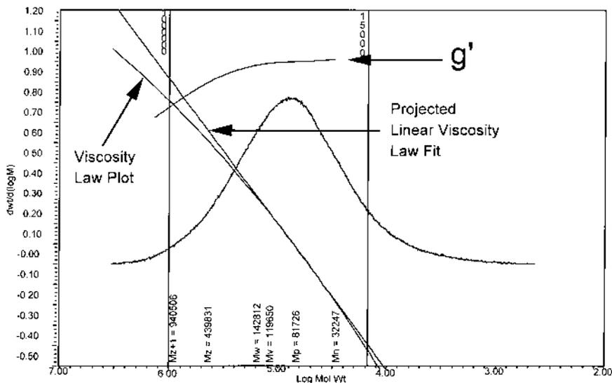
**Figure 19** Molecular-weight distribution and branching information for a low-density polyethylene heavy-wall trash bag. The decrease in branching index,  $g'$ , indicates that the higher-molecular-weight fractions have significant long-chain branching.
