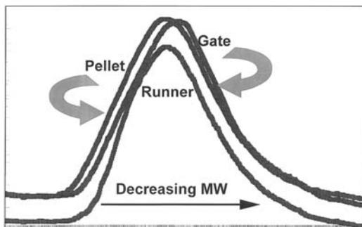
**Figure 1** Injection molding effects. Solvent: 1,2,4-trichlorobenzene. Temperature: 140°C. Columns: Styragel HT6, HT5, HT4, and HT3. The shift in the molecular-weight distribution of the “Gate” sample may be due to melt shear-induced reduction of the largest molecules after passing through the mold gate.
