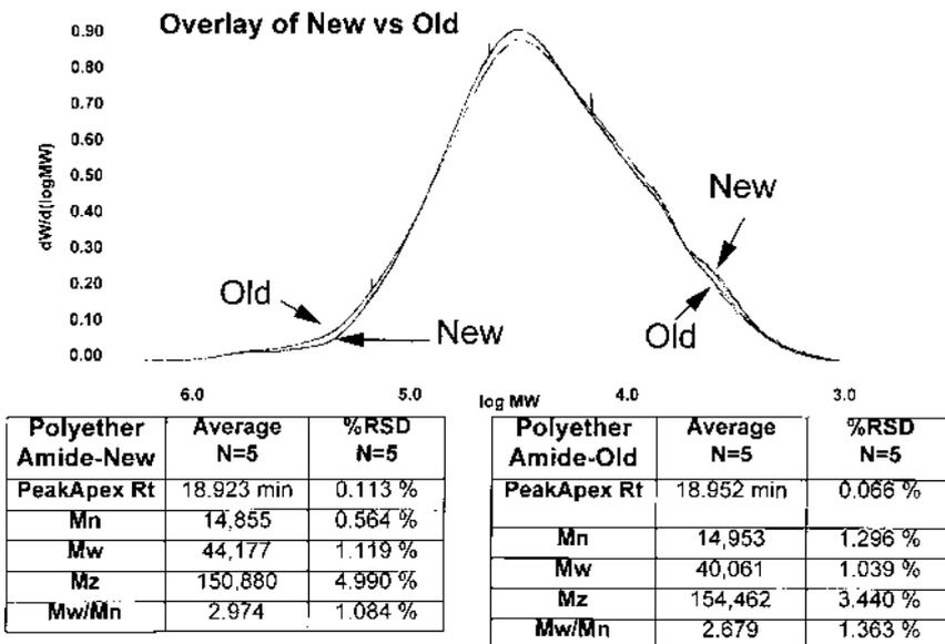
**Figure 17** Alliance narrow-bore GPC (medical, pastic-grade polyether amide). Very subtle differences in the molecular-weight distributions are determined reliably with modern, high-performance instrumentation. Each chromatogram is actually an overlay of five consecutive analyses.
