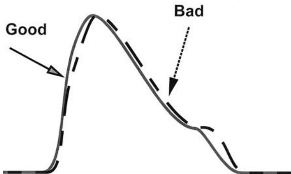
**Figure 3** Comparison of results. Many differences in properties or processability of polymers can be explained by comparing molecular-weight regions. In this example the bad sample has slightly less high-molecular-weight and more low-molecular-weight content than the good sample.
