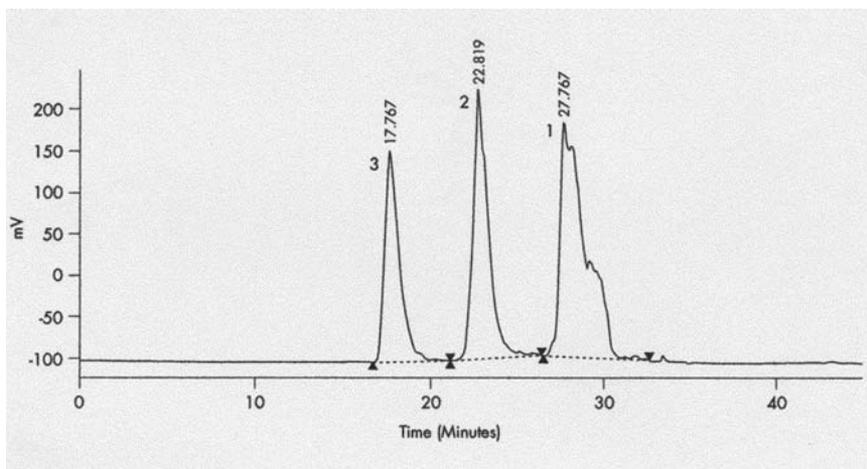
**Figure 20** Chromatogram of poly(methyl methacrylate) 3, poly(styrene) 2 and poly(butadiene) 1. Chromatographic conditions: 30-min. linear gradient, 100% methanol to 100% tetrahydrofuran at 1 mL/min. NovaPak Cyano-Propyl  $3.9 \times 75$  mm,  $4\text{-}\mu\text{m}$  column at  $30^\circ\text{C}$ , evaporative light-scattering detector.
