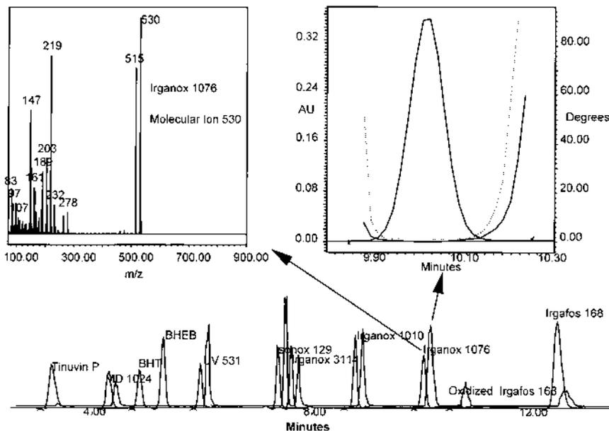
**Figure 14** Additive analysis results. The chromatogram is an overlay of the MS and PDA responses. Each response curve contains extraordinary amounts of information. The mass spectrum, upper left, and a spectral measure of peak purity, upper right, have been extracted from the chromatogram. — TMD: total ion chromatogram from 100 to 700 amu. . . PDA: extracted chromatogram at 230 nm.
