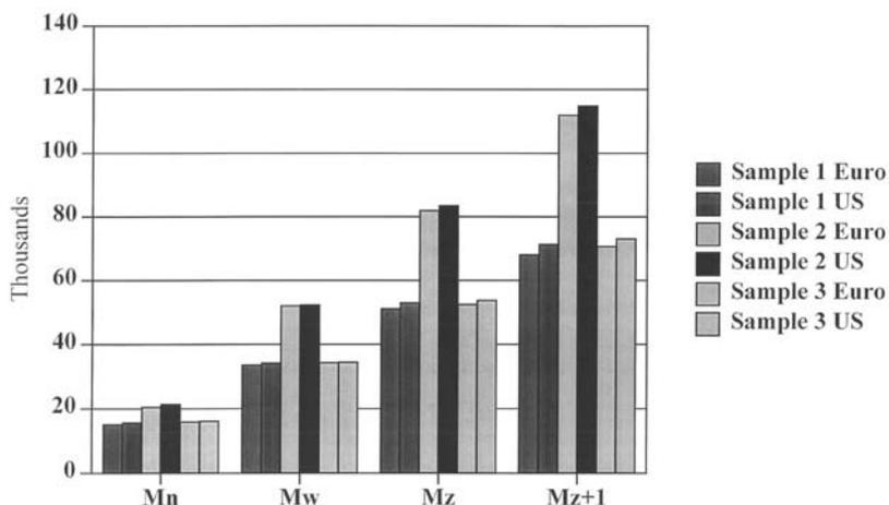
**Figure 18** Alliance GPC interlaboratory results (polycarbonates). Reproducibility within labs and accuracy of results, as measured by the agreement between labs, was exceptional, despite slightly different operating conditions.
