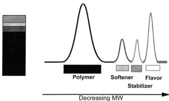
**Figure 2** GPC example: chewing gum. The chromatogram is not to scale—the stabilizer and flavor peaks would probably be much smaller and would consist of one or more monodisperse peaks instead of the distribution shown to illustrate the size separation concept.
