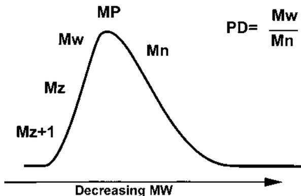
**Figure 7** The calculated molecular-weight values correspond to regions of the full distribution. The peak molecular weight,  $M_p$ , is not calculated but read directly from the chromatogram. The polydispersity,  $PD$ , is the ratio of the weight-average to number-average molecular-weight, an indication of the broadness of the molecular-weight distribution.
