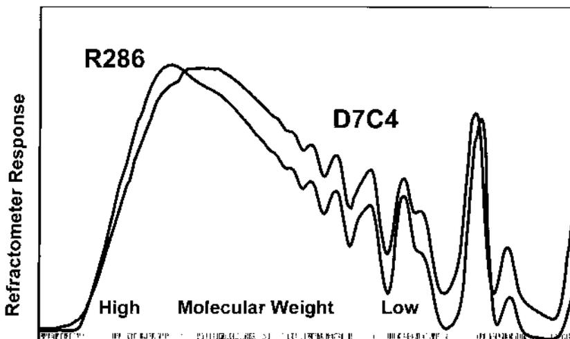
**Figure 4** Phenolic resins from different vendors. GPC is useful for incoming quality control, technical support, and competitive analysis. Differences in the molecular-weight distributions of these two phenolic resins could correspond to acceptable and unacceptable processability or performance.
