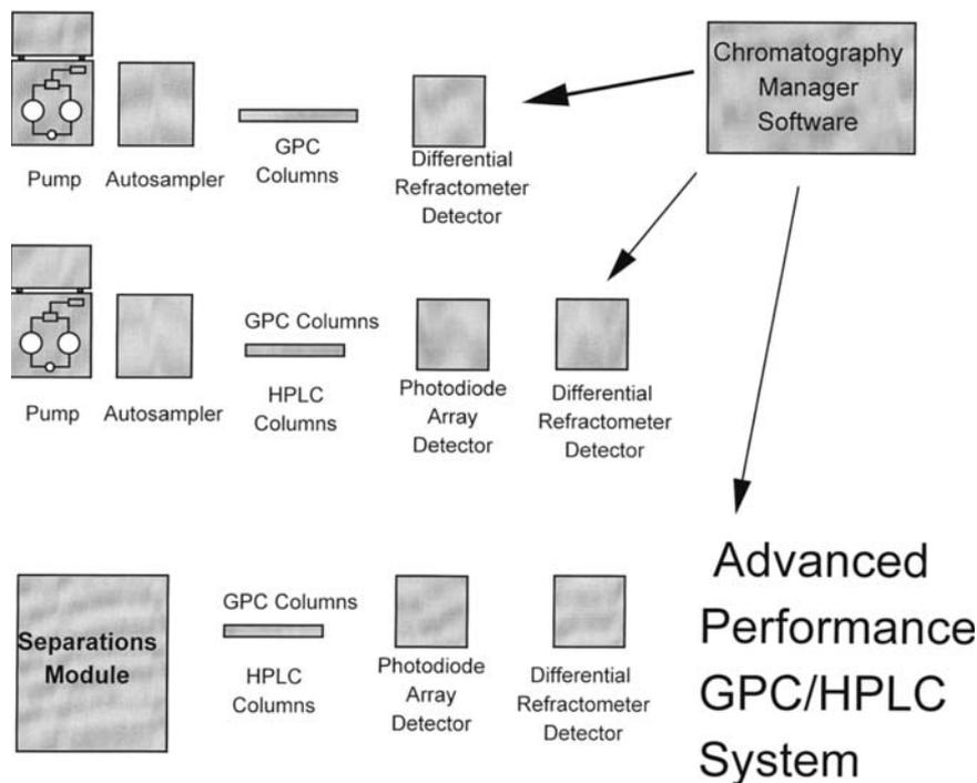
**Figure 8** Primary components of modern GPC/HPLC instruments.
