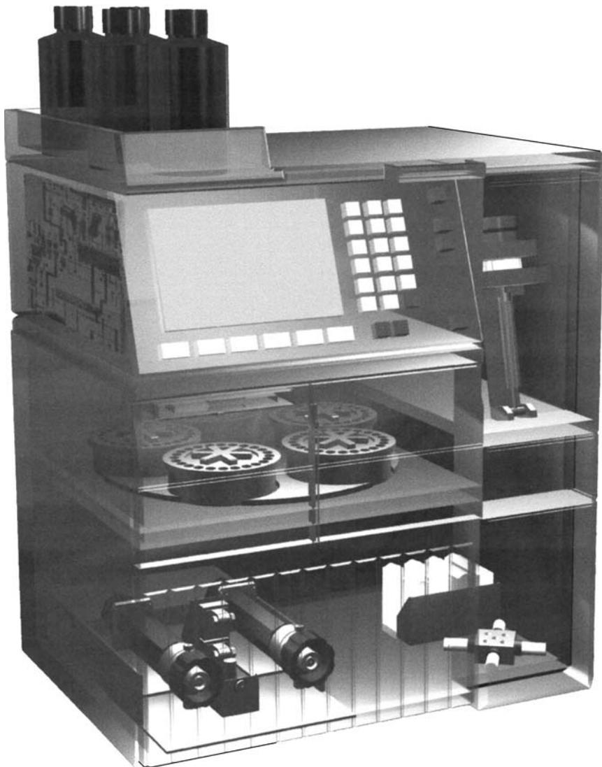
**Figure 10** The primary components of the system shown in [Fig. 9](#) include the control panel (upper left), injection mechanism (upper right), auto-sampler carousels (mid-level), independently driven dual reciprocating solvent delivery pistons (lower left), and degasser/solvent select module (lower right).
