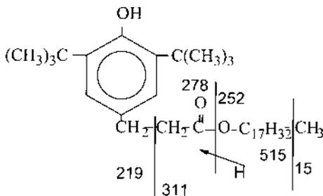
**Figure 15** The classical electron impact mass spectra produced enable definitive compound identification, Irganox 1076 in this example. Electron impact mass spectra are interpretable as well as library-searchable.
