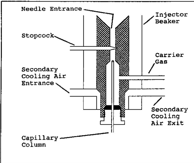
**Figure 4** On-column injector.
