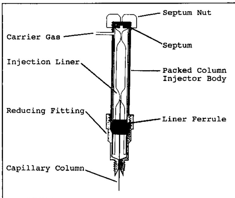
**Figure 5** Direct injector.
