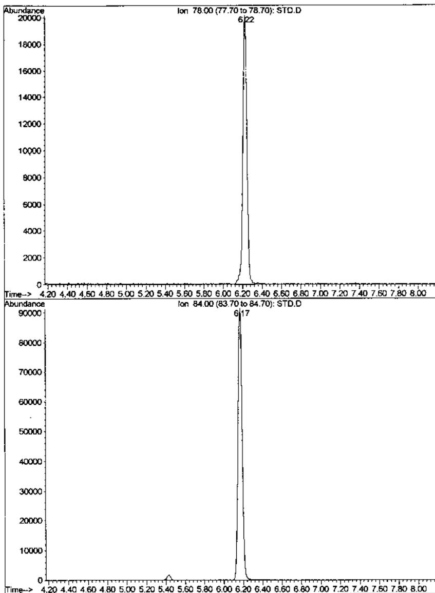
**Figure 8** GC chromatogram: trace analysis of benzene in polymer by purge-and-trap GC-MS. The single-ion signal for benzene ( $m/z$ , 78) is displayed on top, while the single-ion signal for deuterated benzene ( $m/z$ , 84) is displayed below.
