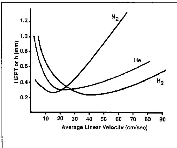
**Figure 6** van Deemter curves for three main carrier gases: N<sub>2</sub>, He, and H<sub>2</sub>.
