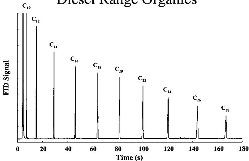
**Figure 13** GC chromatogram illustrating the high speed of analysis using ChromatoFast technology. (Courtesy of ChromatoFast.)
