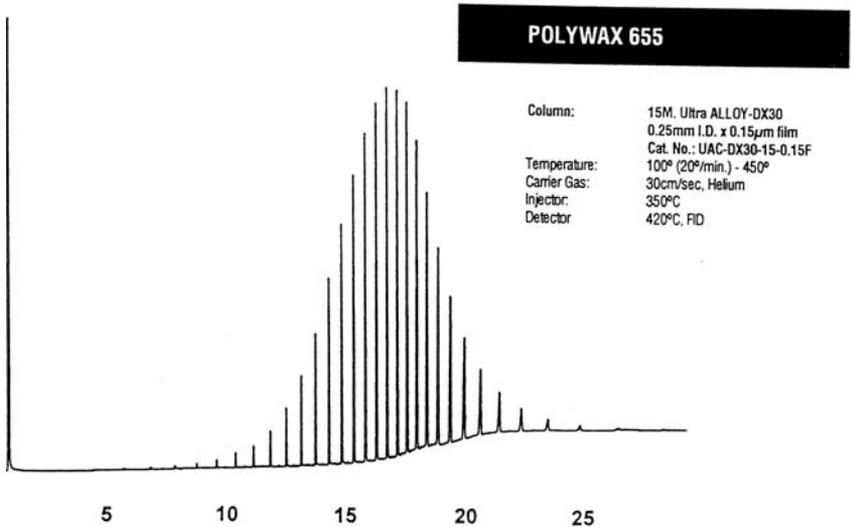
**Figure 10** Analysis of high-molecular-weight waxes, illustrating the power of high-temperature GC columns. Note the high temperature limit for the column and the relatively short retention time. (Courtesy of Quadrex Corporation.)
