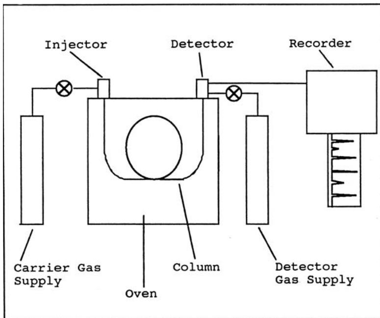
**Figure 1** General diagram of a gas chromatograph.
