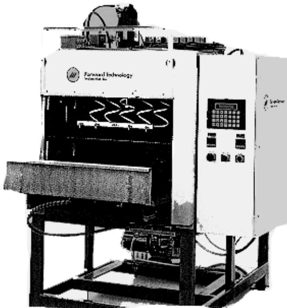
Figure 1.5 A typical vertical platen hot tool welder .
