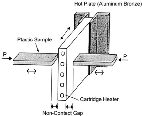
**Figure 1.4.** Non-contact hot plate welding. Parts being welded are placed near the hot plate, separated from it by a distance referred to as the non-contact gap. The hot plate is removed during the change-over phase, and pressure is applied to hold the parts in intimate contact during weld cooling and solidification.
