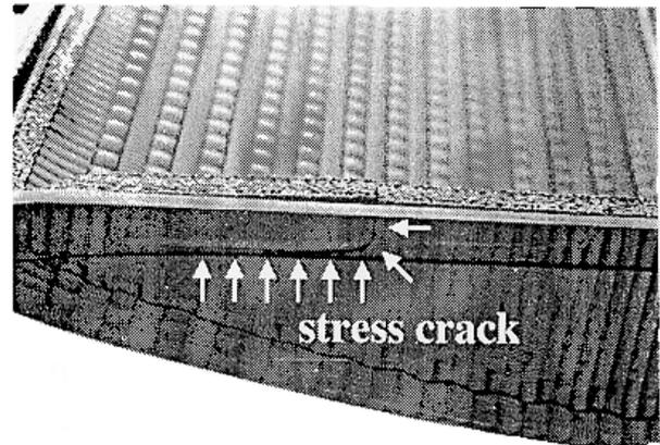
**Figure 1.8** Stress cracking in tail lights. Welding induces internal stresses which later cause cracks to form.
