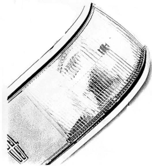
**Figure 1.7** An automobile headlight; parts were joined using hot tool welding.
