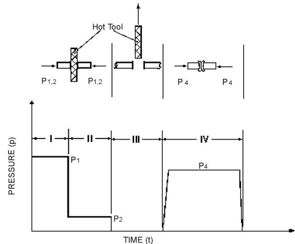
**Figure 1.2** Pressure vs. time curve showing the four phases of heated tool welding. Parts to be welded are pressed against the hot tool in phase I, and heat is transferred to the parts by conduction. Melting begins when the melt temperature of the plastic is reached. In phase II, pressure is reduced in order to increase melt thickness. In phase III, the hot tool is removed, and in phase IV, the parts are brought together under pressure to cool and solidify.
