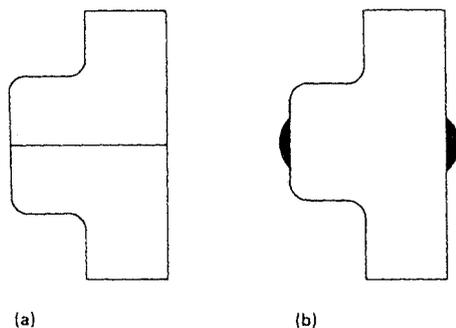
**Figure 1.1** A butt joint used for hot tool welding, shown before and after welding.
