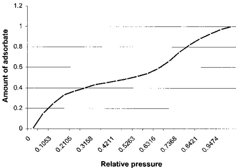
FIG. 4.4 Adsorption isotherm curve-type 4.
