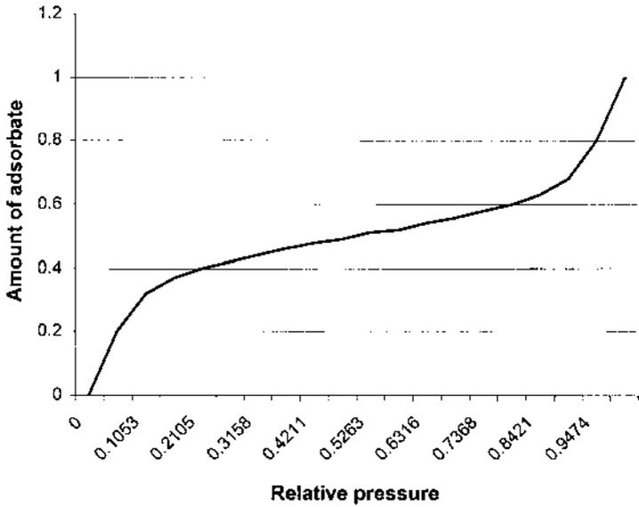
**FIG. 4.2** Adsorption isotherm type 2 (BET) on homogeneous adsorbent.
