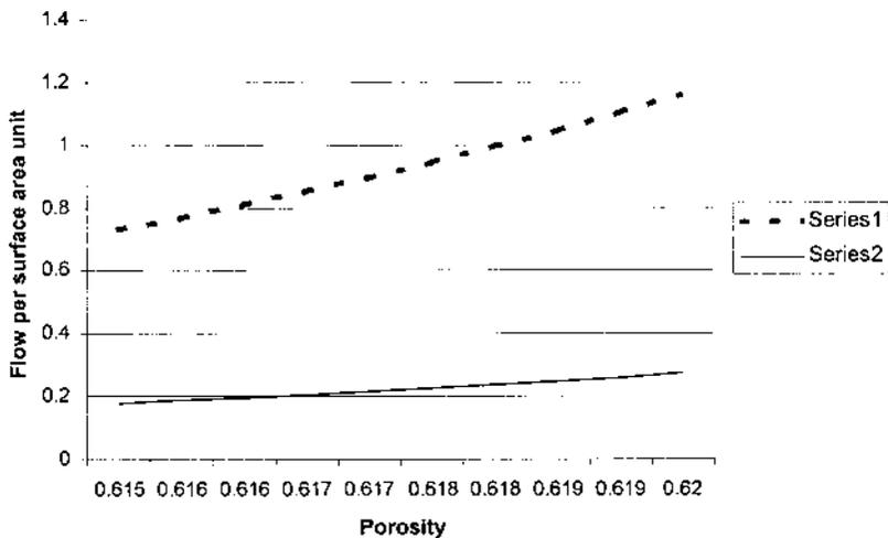
**FIG. 4.16** Mass-transfer for heterogeneous catalysis: appearance of VPT for varied coordination number: Series 1:  $n_n = 6$ , Series 2:  $n_n = 4$ .
