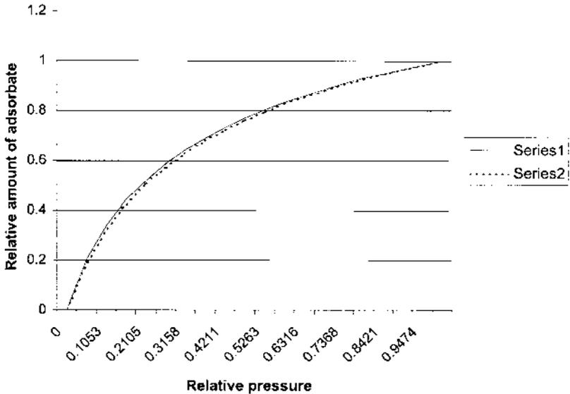
**FIG. 4.10** Relative amount of adsorbate vs. relative pressure under varied temperatures. Series 1: Temperature 300 K; Series 2: Temperature 389 K.
