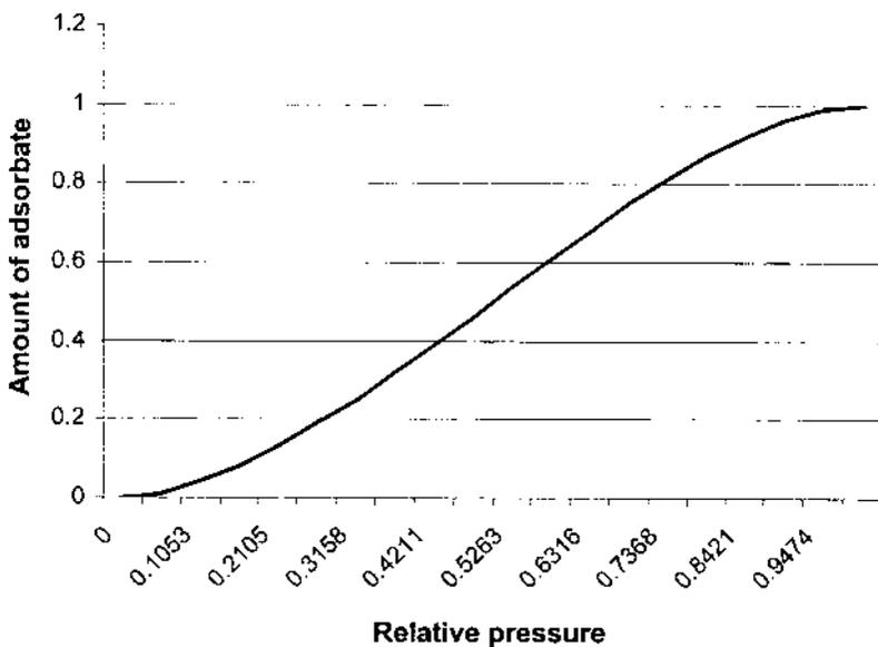
FIG. 4.5 Isotherms of adsorption: type 5.
