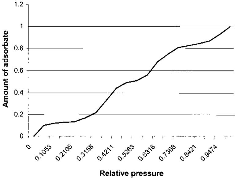
**FIG. 4.6** Type 6 of adsorption isotherms.
