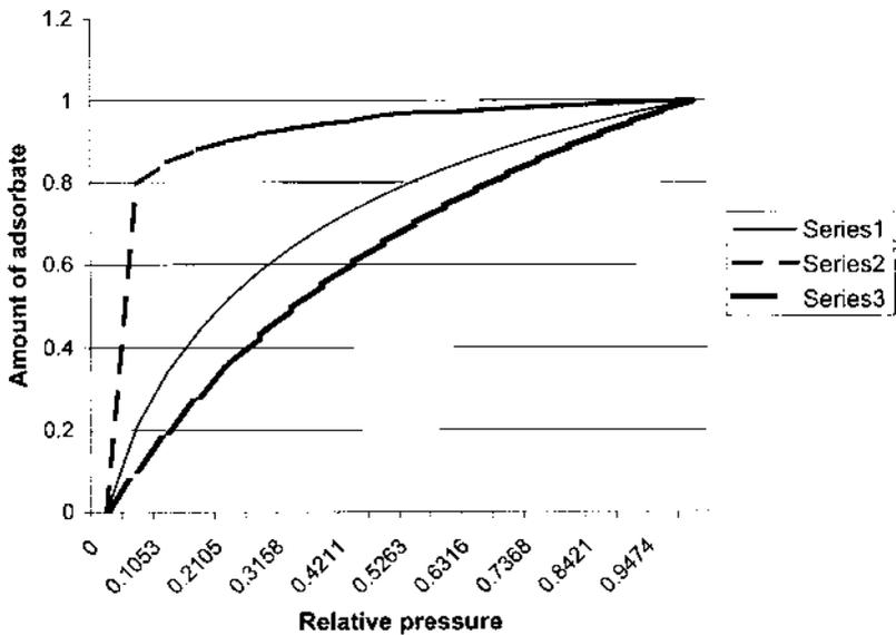
**FIG. 4.8** Langmuir-like approach for micropores, adsorption isotherm curves: Series 1:  $\gamma_p = 1$ ; Series 2:  $\gamma_p = 10$ ; Series 3:  $\gamma_p = 0.1$ .
