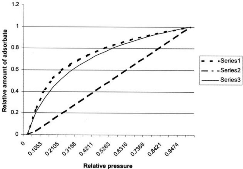
**FIG. 4.9** Forms of Dubinin, Langmuir-like, and mixed (intermediary) adsorption isotherm curves: Series 1: Isotherm adsorption curve built according to VFMT; Series 2: Mixed (intermediary) curve built on the base of the combination of condensation approximation with Gibbs energy distribution; Series 3: Langmuir-like curve.
