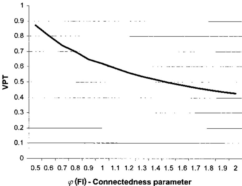
**FIG. 4.17** Permeability as function of connectedness for sphere.
