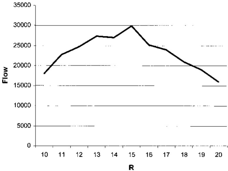
**FIG. 4.21** Influence of the exterior radius on the total flow through the total exterior surface.
