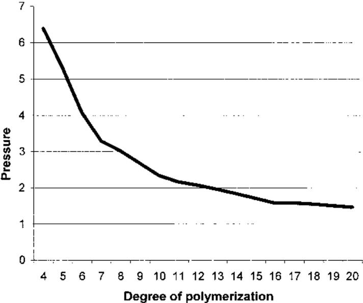
**FIG. 4.22** Pressure needed for additional cross-linking in macromolecules (number of branching  $m = 5$ ).
