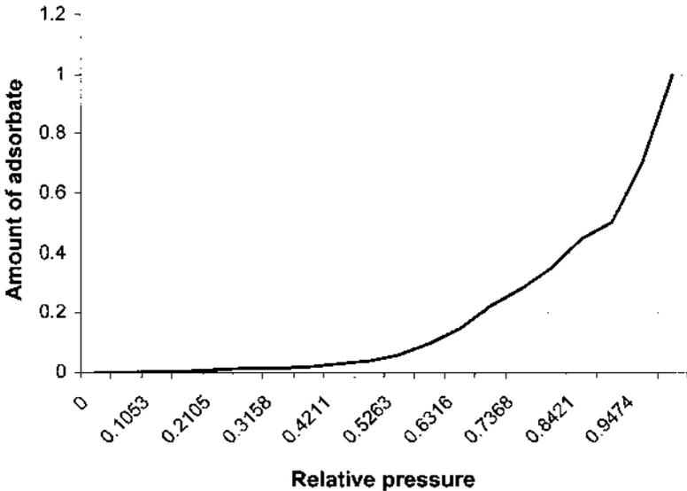
**FIG. 4.3** Type 3 of adsorption isotherm curves.
