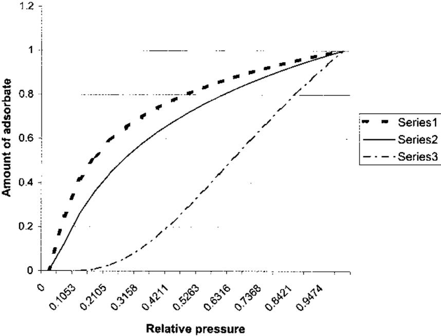
**FIG. 4.7** Adsorption isotherm curves in VFMT: Series 1:  $b_a = 1/(10R_gT)^2$ ; Series 2:  $b_a = 1/10/(R_gT)^2$ ; Series 3:  $b_a = 1/(R_gT)^2$ .
