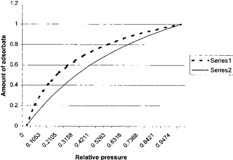
**FIG. 4.1** Adsorption isotherm type 1 (Langmuir) for gas on homogeneous adsorbent. Series 1: microporous adsorbent; Series 2: external surface.
