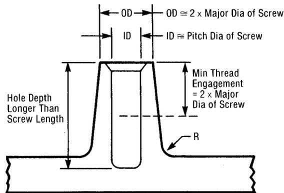
**Figure 68.4:** Boss design guidelines for self tapping screws, Dylark styrene maleic anhydride copolymer.
