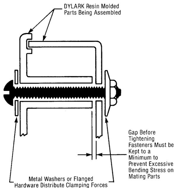
**Figure 68.2:** Bolted assembly, Dylark styrene maleic anhydride copolymer.
