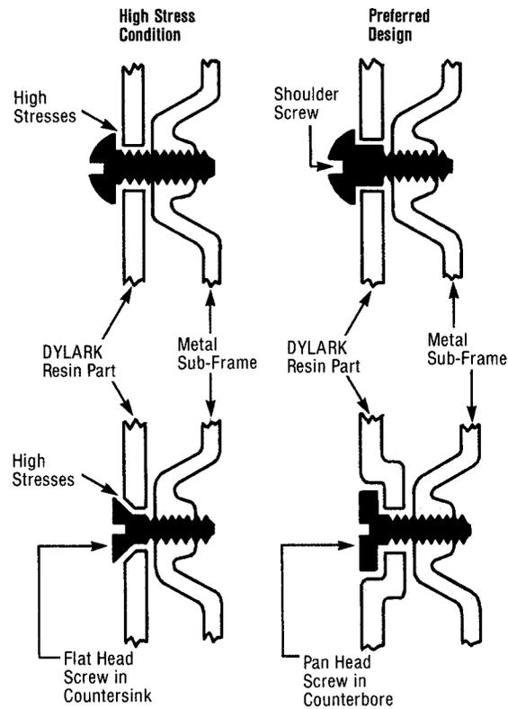
**Figure 68.3:** Managing stress levels in the plastic part when assembly torque cannot be controlled, Dylark styrene maleic anhydride copolymer.
