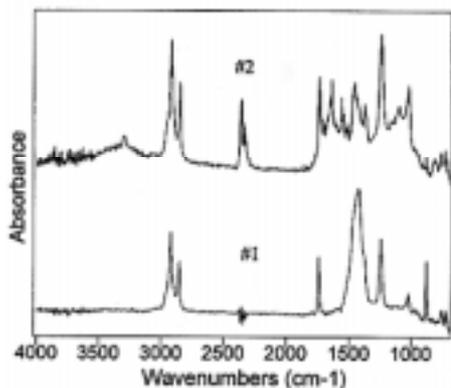
Figure 8. Micro IR reflectance spectra of EVA hot melt adhesive - #1 unfused pellets; #2 dark brown adhesive from heated reservoir.
