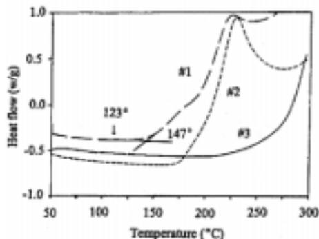
Figure 6. DSC-OI temperature of same samples as in Figure 5 - see Table 1 for initial onset and extrapolated OI temperatures. Values are shown for #1. 123° initial onset and 147° extrapolated.
