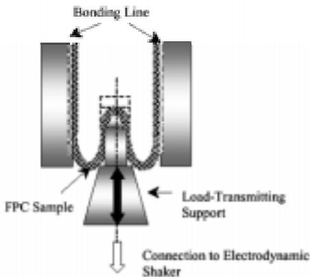
Figure 1. General schematic of load-transmitting support.
