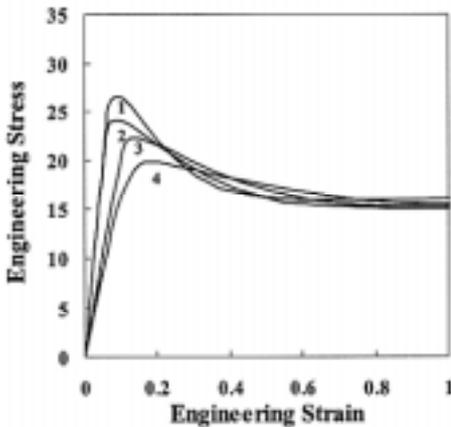
Figure 1. Stress-strain diagrams of PE 100 HDPE ramp test at strain rates. 1 -  $\dot{\epsilon} = 0.33 \text{ s}^{-1}$ , 2 -  $\dot{\epsilon} = 0.033 \text{ s}^{-1}$ , 3 -  $\dot{\epsilon} = 0.0033 \text{ s}^{-1}$ , 4 -  $\dot{\epsilon} = 0.00033 \text{ s}^{-1}$ .
