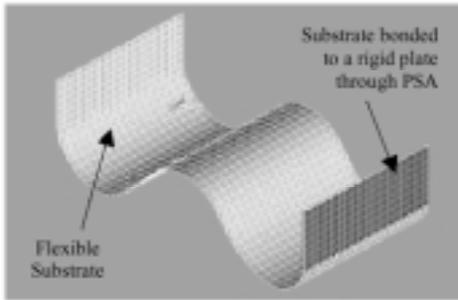
Figure 3. The Finite Element Analysis (FEA) model.
