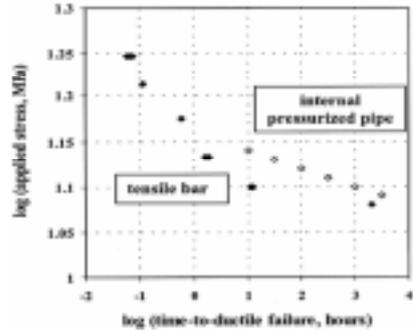
Figure 3. Time-to-necking and -to-ductile failure vs. applied stress (HDPE: BG10050).
