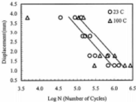
Figure 2. S-N (D-N) diagram for material system A.
