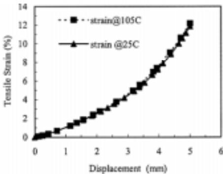
Figure 5. The FEA data: tensile stress versus displacement.
