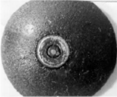
Figure 4. EPDM hot water check valve molded on metal support. Surface is degraded and uneven; metal spring in center has broken through the degraded EPDM. Overall diameter is approx. 5/8 inch (20 mm).
