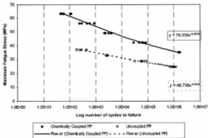
Figure 1. The variation of maximum fatigue stress of CCPP and UCPP with the number of fatigue cycles (Wohler curves).
