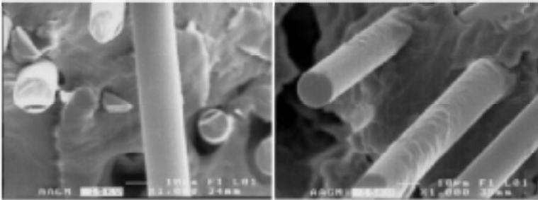
Figure 4. Fiber surfaces in FA (left) and in FFA (right) of naturally fatigued of CCPP at 1000 magnifications.
