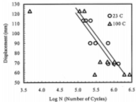
Figure 6. S-N diagram for material system A constructed based on experimental and FEA data.
