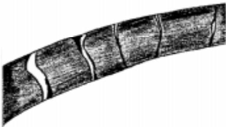
Figure 1. HDPE power cable jacket fractured by oxidative degradation due to water and copper in contact with jacket. Copper below jacket shows through cracks.
