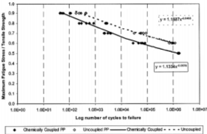
Figure 2. The variation of normalized of maximum fatigue stress of CCPP and UCPP with the number of fatigue cycles (normalized Wohler curves).
