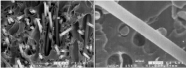
Figure 5. Fracture surfaces in elastic deformation portion of unfatigued UCPP at 200 magnifications (left) and fiber surface in FFA of naturally fatigued of UCPP at 1000 magnifications (right).
