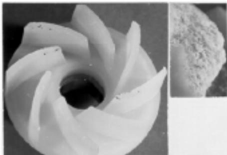
Figure 2. Unused PP rotor and closeup of a degraded fin of a used rotor.
