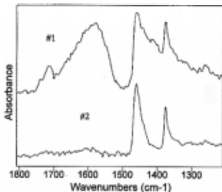
Figure 7. Micro IR reflectance spectra of EPDM valve - #1 degraded outer surface - bound oxygen at 1500-1800  $\text{cm}^{-1}$  not present below surface; #2 inner bulk below degraded outer surface.
