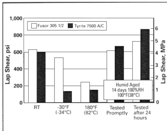
**Figure 34.2:** Lap shear bond strengths for Amoco Amodel AS1133HS 33% glass fiber reinforced PPA resin. (Fusor 305-1/-2 is a two part epoxy adhesive. Tyrite 7500 A/C is a two part urethane adhesive. Both adhesives are supplied by Lord Corporation).
