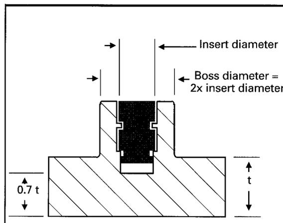
**Figure 34.1:** Boss design for ultrasonic inserts in Amodel PPA resin.
