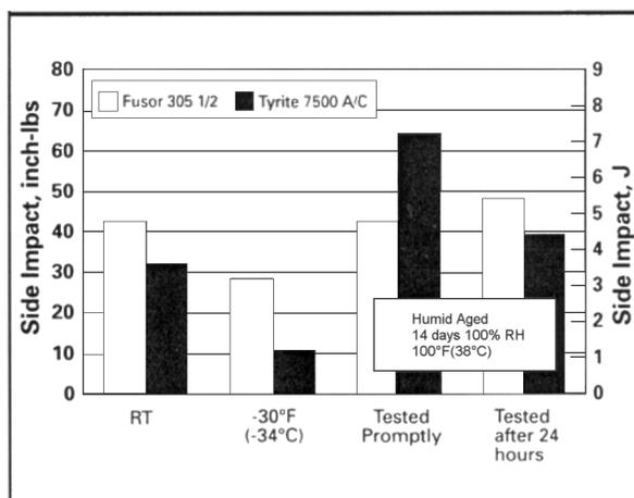
**Figure 34.3:** Side impact bond strengths for Amoco Amodel AS1133HS 33% glass fiber reinforced PPA resin. (Fusor 305-1/-2 is a two part epoxy adhesive. Tyrite 7500 A/C is a two part urethane adhesive. Both adhesives are supplied by Lord Corporation).
