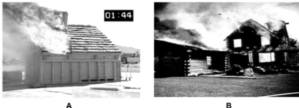
Figure 5. Polypropylene swamp cooler 1 minute and 44 seconds after ignition from an external flame source (A). The lack of flame retardant in this product lead to the house fire shown in B.
