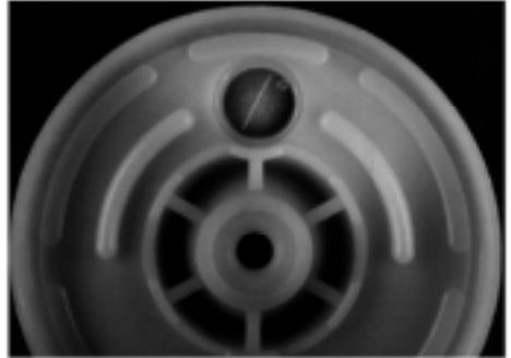
Figure 3. Top view of pressure relief device.
